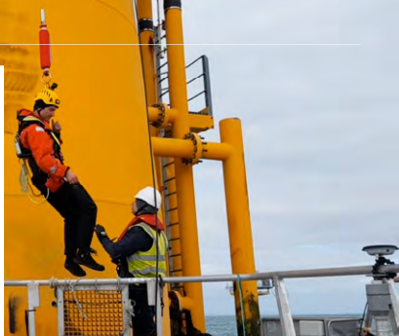
Pict Offshore has been set up to commercialise the 'Get Up Safe' (GUS) system, a motion compensated personnel hoist
